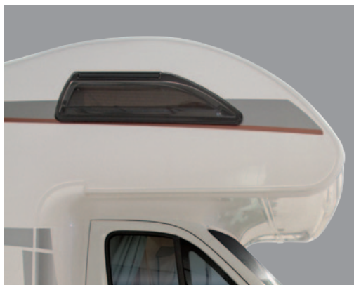
Seitz living compartment window with polyurethane frames.
