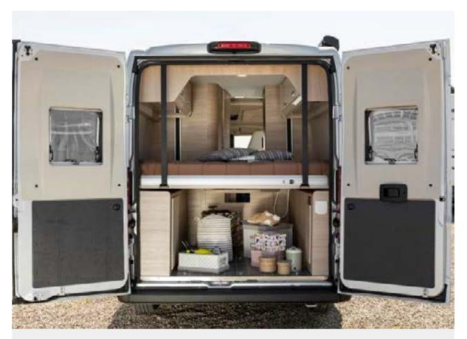
With the electronically-operated rear bed supported by straps, that stops where you want it to, the E-VAN DUO XL offers you a rear stowage compartment with a variable volume of between 1,500 and 2,400 litres.
