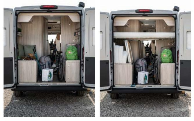
Liftable or removable bed bases to manage stowage space as needed.
