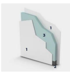
Roof by a double sheet of fiberglass, external and internal, PVC chassis and waterproof plastic inserts, thickness 30 cm.
