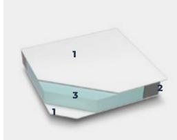
Wall with double sheet of fiberglass, external and internal, PVC frame and waterproof plastic inserts, thickness 30 cm.
